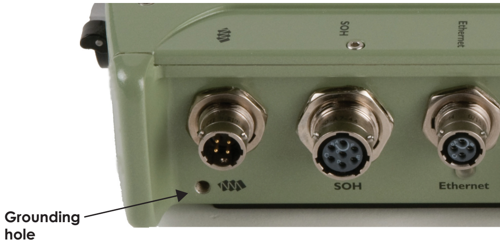
Figure 4-2 Hole for grounding lug screw
